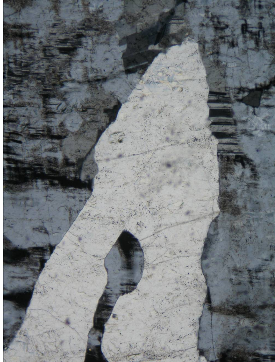
Quartz and feldspars in a graphic intergrowth in pegmatite from Maršíkov, the Czech Republic; PPL (left) and XPL (right). Width of fields of view is ca. 1.5 mm. Photo: JiZi.
