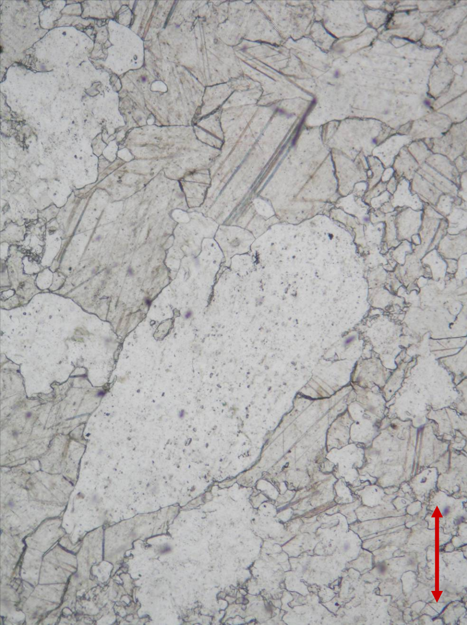
Quartz with laminar undulatory extinction in marble from Heřmanovice, the Czech Republic; PPL (left) and XPL (right). Width of fields of view is ca. 1.8 mm. Photo: JiZi.
