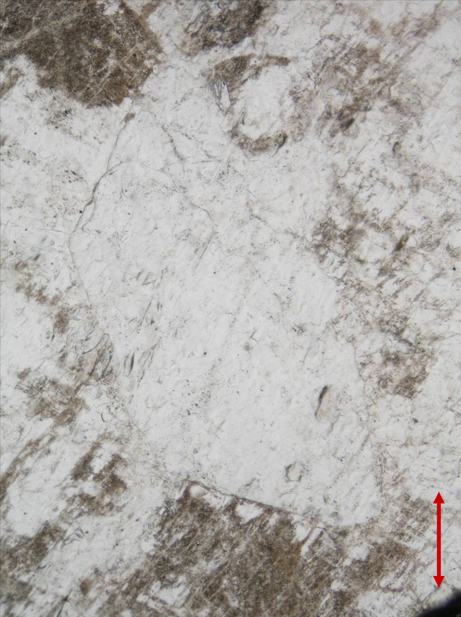
Undulatory quartz with feldspars in pegmatite from Maršíkov, the Czech Republic; PPL (left) and XPL (right). Width of fields of view is ca. 1.5 mm. Photo: JiZi.
