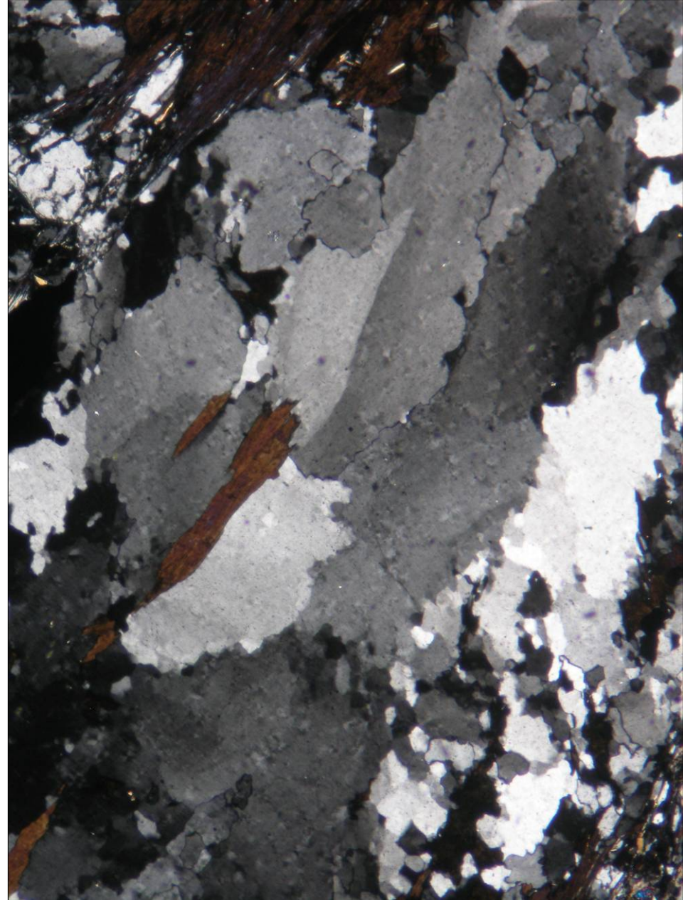
Quartz in quartzite from Zlaté Hory, the Czech Republic; PPL (left) and XPL (right). Width of fields of view is ca. 1.8 mm. Photo: JiZi.
