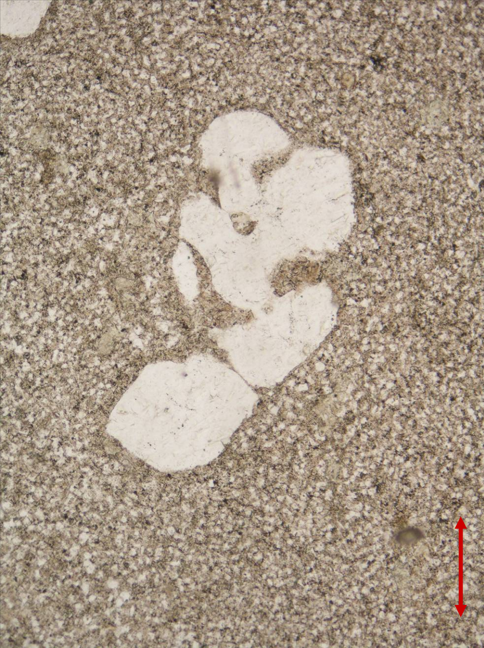
Embayed quartz phenocrysts in palaeorhyolite from Teplice, the Czech Republic; PPL (left) and XPL (right). Width of fields of view is ca. 1.5 mm. Photo: JiZi.
