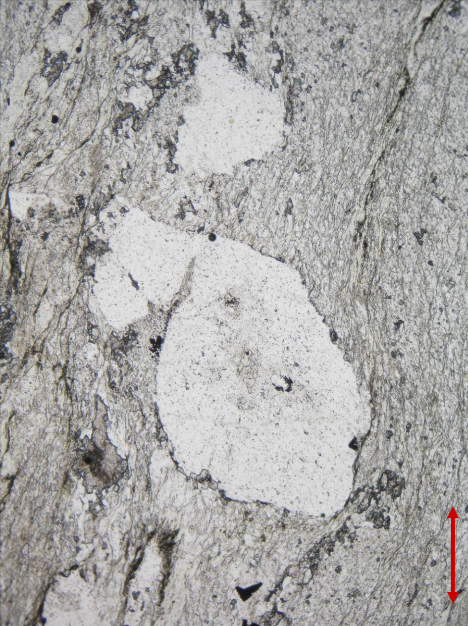
Quartz phenocrysts in metamorphosed palaeorhyolite from Oskava, the Czech Republic; PPL (left) and XPL (right). Width of fields of view is ca. 1.8 mm. Photo: JiZi.
