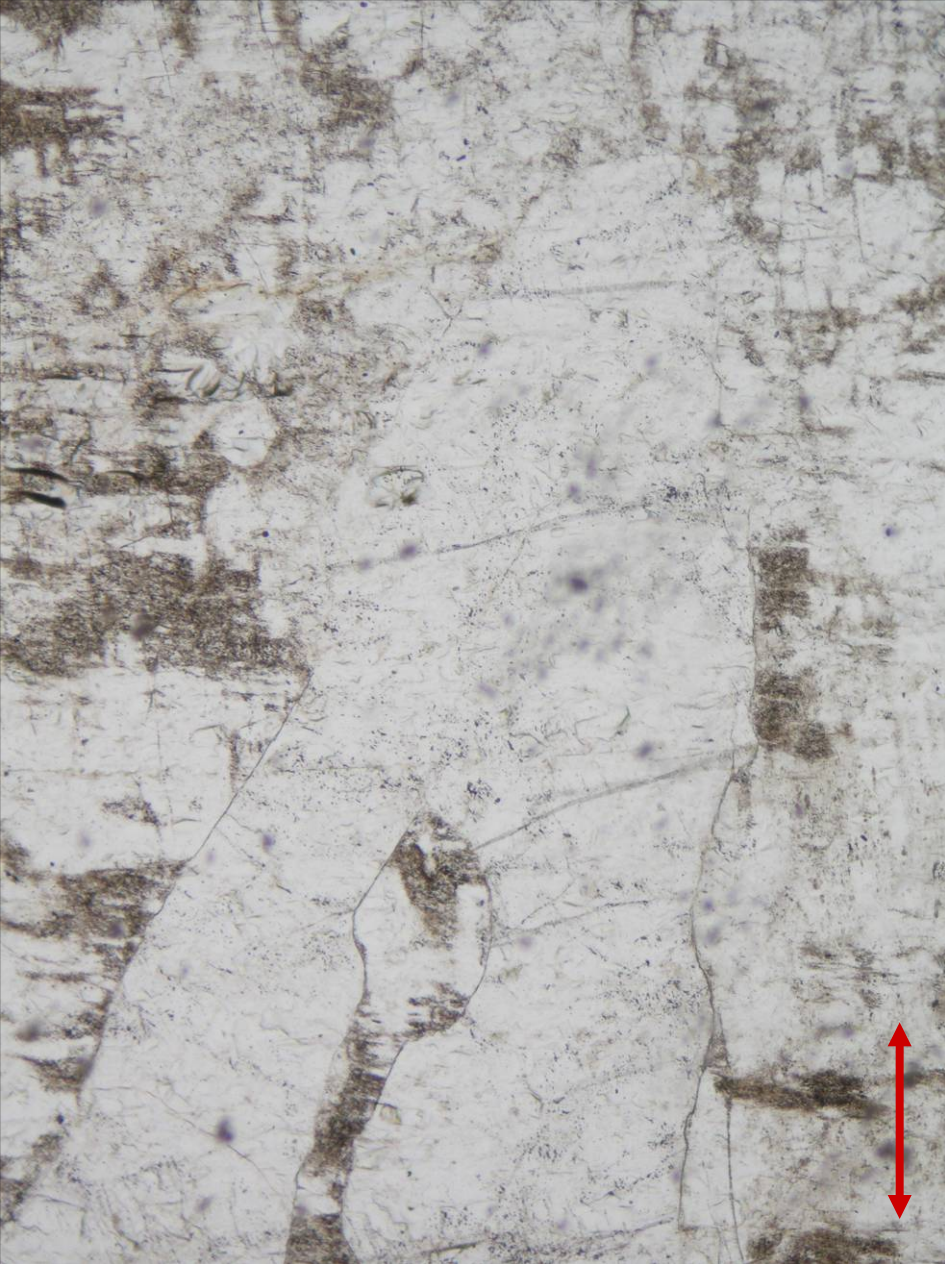
Quartz and feldspars in a graphic intergrowth in pegmatite from Maršíkov, the Czech Republic; PPL (left) and XPL (right). Width of fields of view is ca. 1.5 mm. Photo: JiZi.
