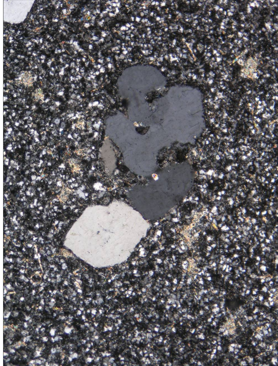
Embayed quartz phenocrysts in palaeorhyolite from Teplice, the Czech Republic; PPL (left) and XPL (right). Width of fields of view is ca. 1.5 mm. Photo: JiZi.
