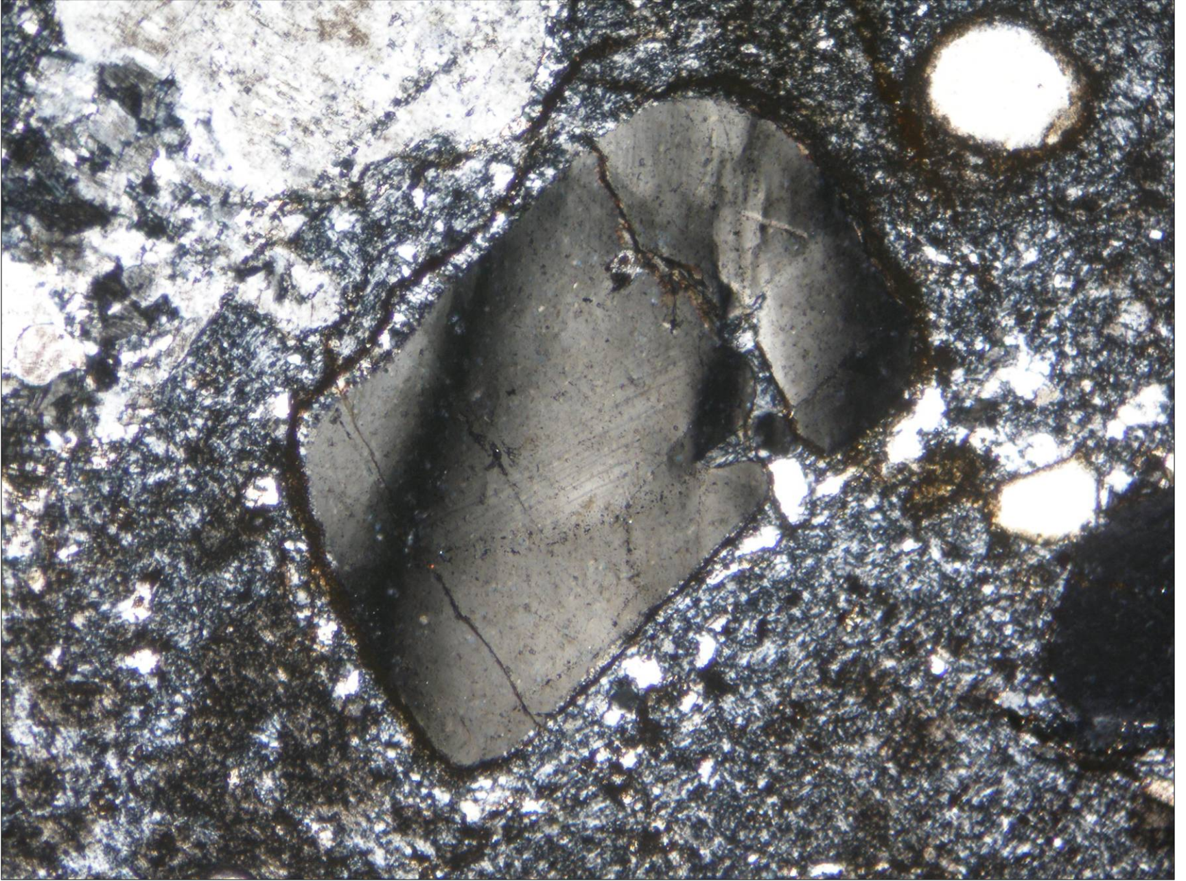
Undulatory quartz in palaeorhyolite from Ludmírov, the Czech Republic; XPL. Field of view is ca. 2.3 mm wide. Photo: JiZi.
