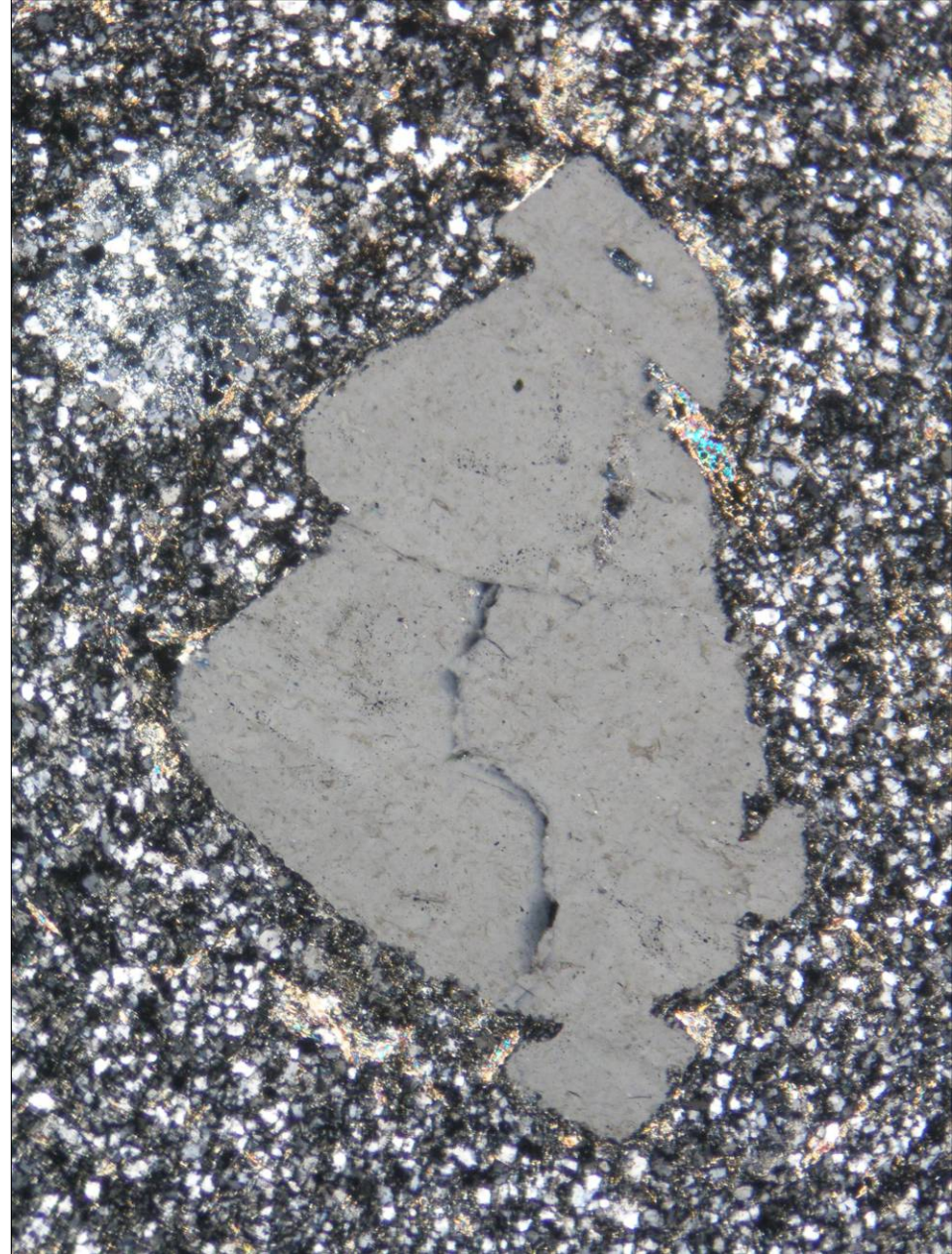
Embayed quartz phenocryst in palaeorhyolite from Teplice, the Czech Republic; PPL (left) and XPL (right). Width of fields of view is ca. 2.0 mm. Photo: JiZi.
