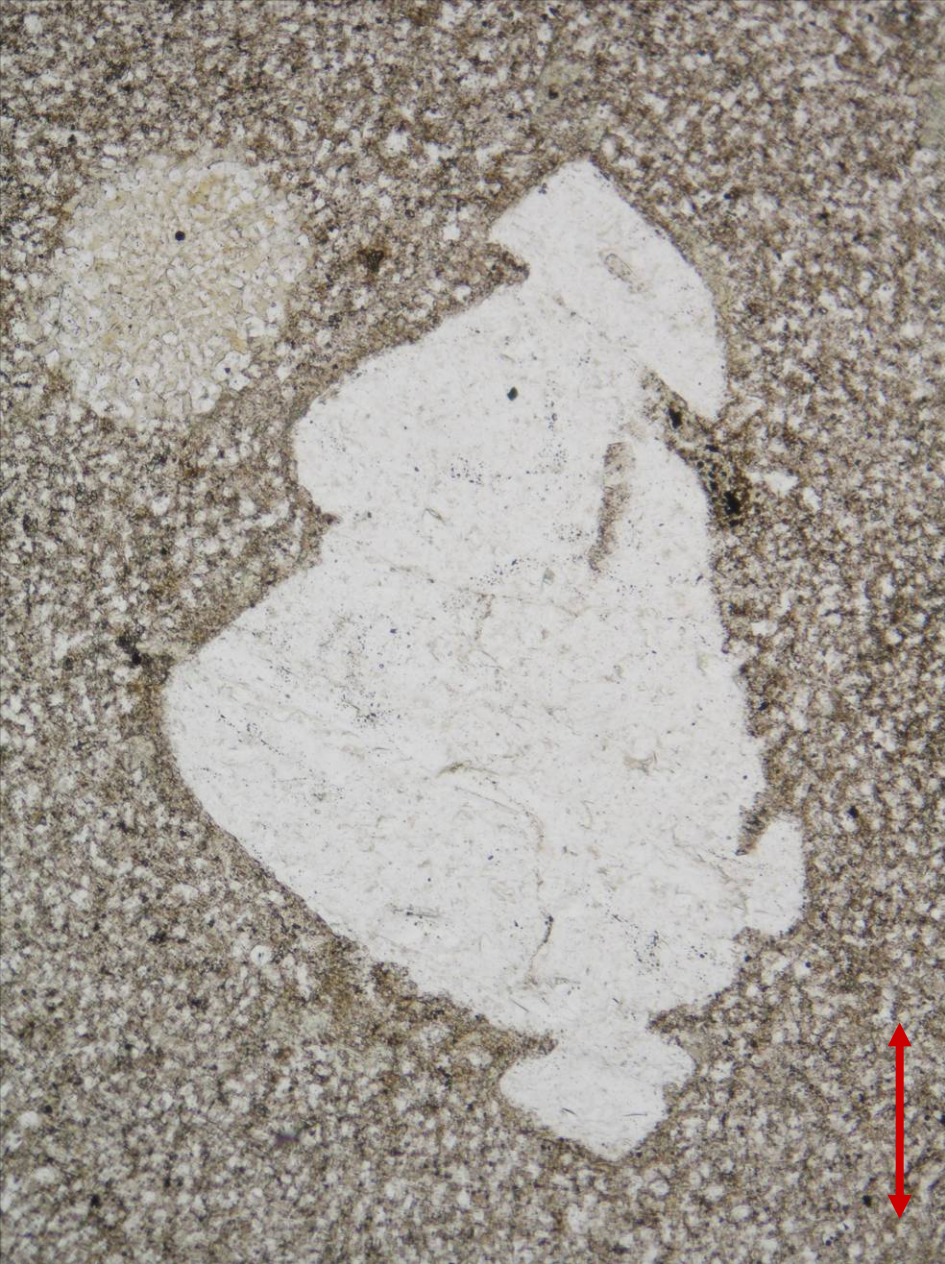
Embayed quartz phenocryst in palaeorhyolite from Teplice, the Czech Republic; PPL (left) and XPL (right). Width of fields of view is ca. 2.0 mm. Photo: JiZi.
