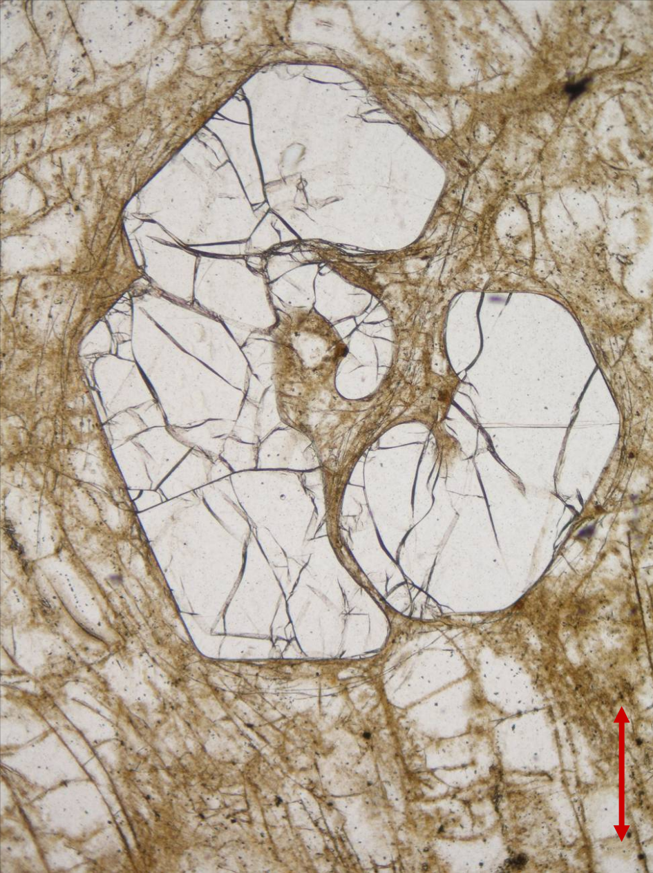
Embayed quartz phenocryst in pitchstone from Triebitschtal near Meissen, Germany; PPL (left) and XPL (right). Width of fields of view is ca. 1.5 mm. Photo: JiZi.
