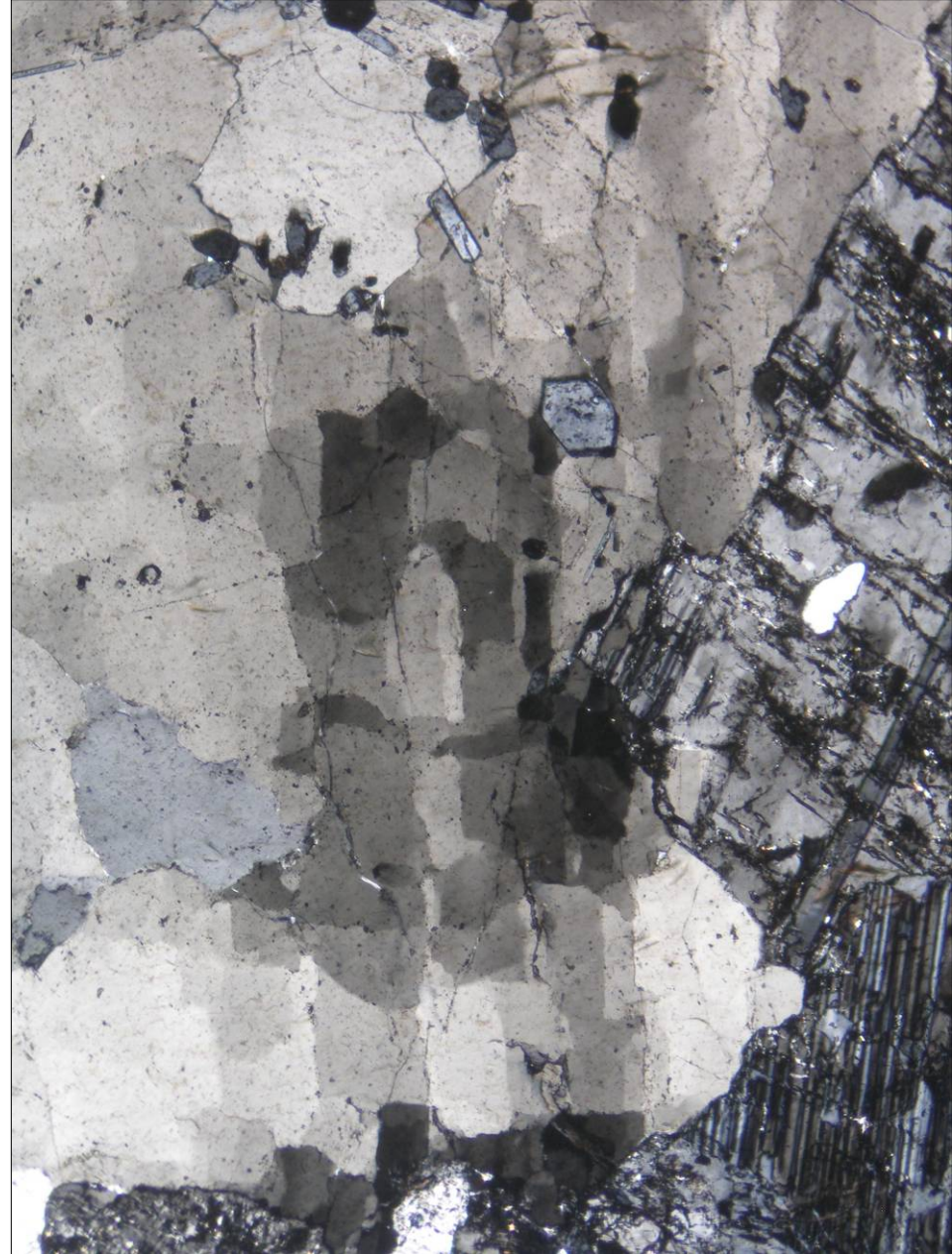
Quartz in pegmatite from Žulová, the Czech Republic; PPL (left) and XPL (right). Width of fields of view is ca. 1.7 mm. Photo: JiZi.
