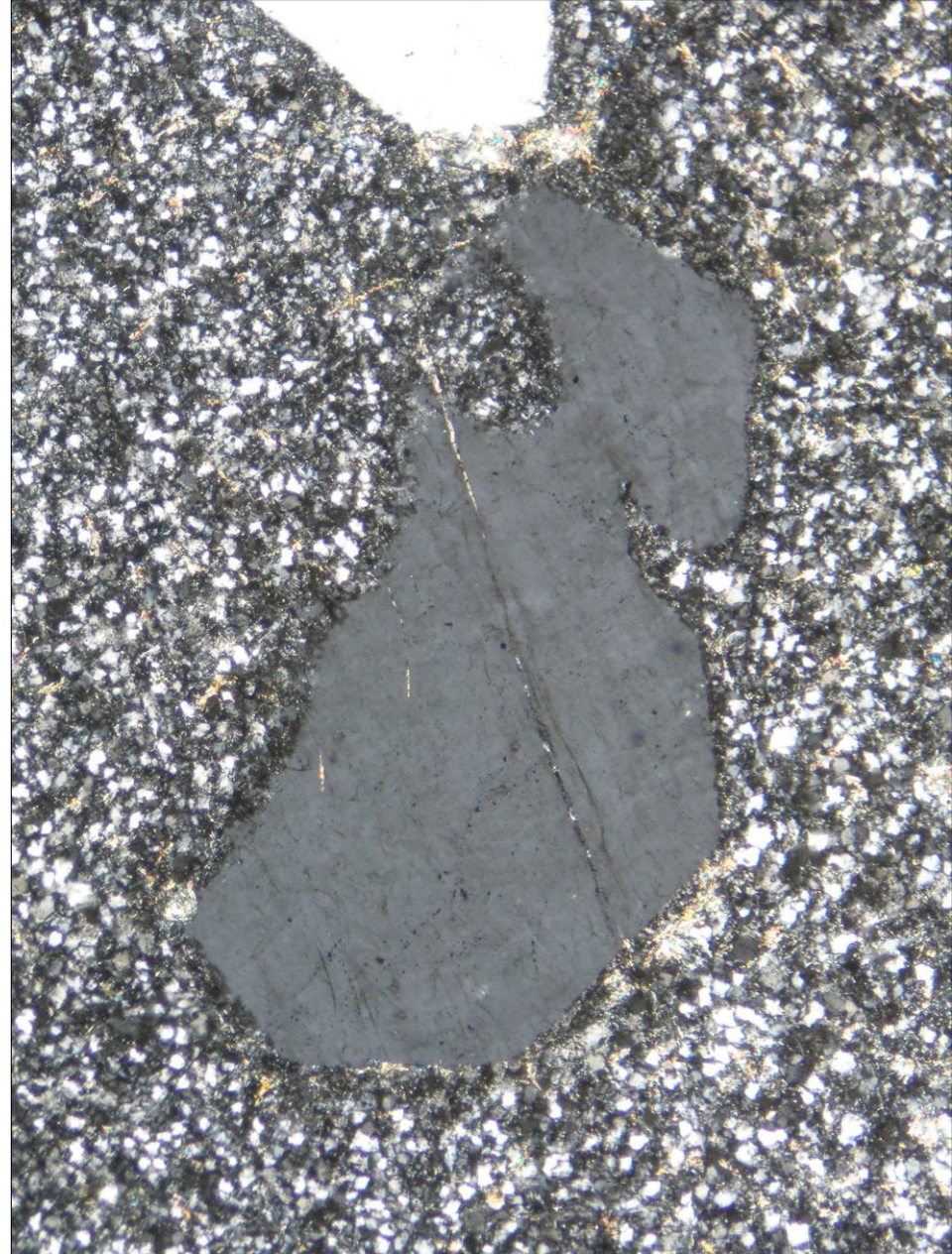
Embayed quartz phenocryst in palaeorhyolite from Teplice, the Czech Republic; PPL (left) and XPL (right). Width of fields of view is ca. 1.5 mm. Photo: JiZi.
