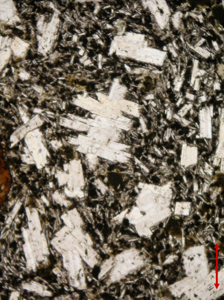
Plagioclase phenocrysts in andesite from Bánov, the Czech Republic; PPL (left) and XPL (right). Width of fields of view is ca. 1.5 mm. Photo: JiZi.
