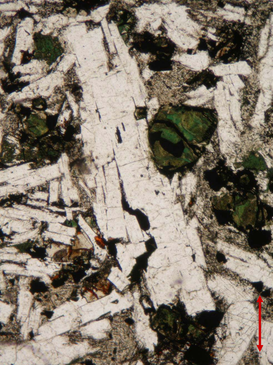
Plagioclase and altered olivine in palaeobasalt from Studenec, the Czech Republic; PPL (left) and XPL (right). Width of fields of view is ca. 1.7 mm. Photo: JiZi.
