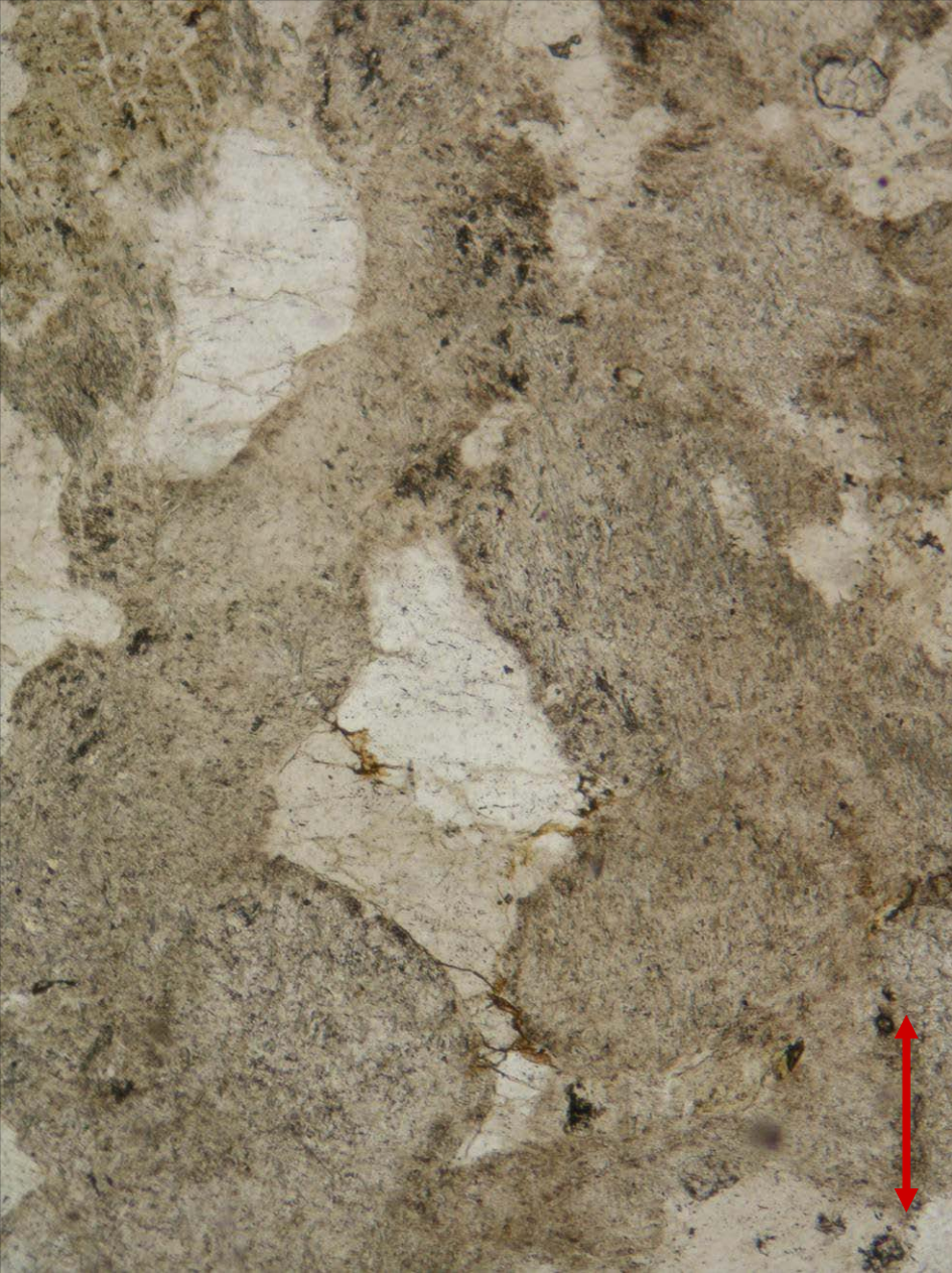
Strongly altered feldspars (mainly plagioclase) and quartz in pegmatite from Supíkovice, the Czech Republic; PPL (left) and XPL (right). Width of fields of view is ca. 1.6 mm. Photo: JiZi.
