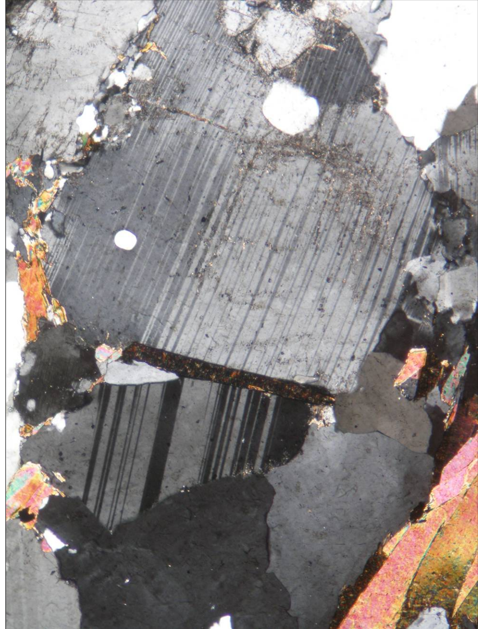
Plagioclase in paragneiss from Dolní Rožínka, the Czech Republic; PPL (left) and XPL (right). Width of fields of view is ca. 1.8 mm. Photo: JiZi.
