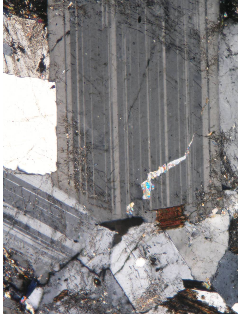
Plagioclase in gneiss from Vanov, the Czech Republic; PPL (left) and XPL (right). Width of fields of view is ca. 1.8 mm. Photo: JiZi.
