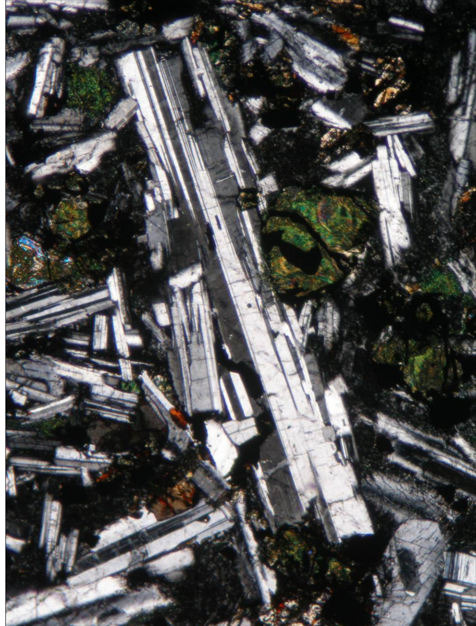
Plagioclase and altered olivine in palaeobasalt from Studenec, the Czech Republic; PPL (left) and XPL (right). Width of fields of view is ca. 1.7 mm. Photo: JiZi.
