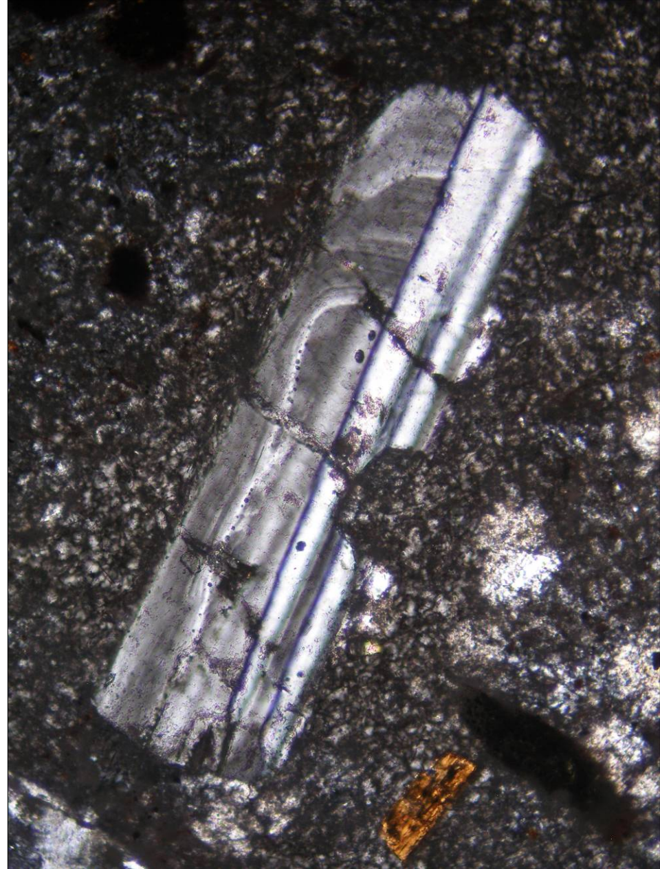
Plagioclase phenocryst in rhyolite from Žiar nad Hronom, Slovakia; PPL (left) and XPL (right). Width of fields of view is ca. 0.7 mm. Photo: JiZi.
