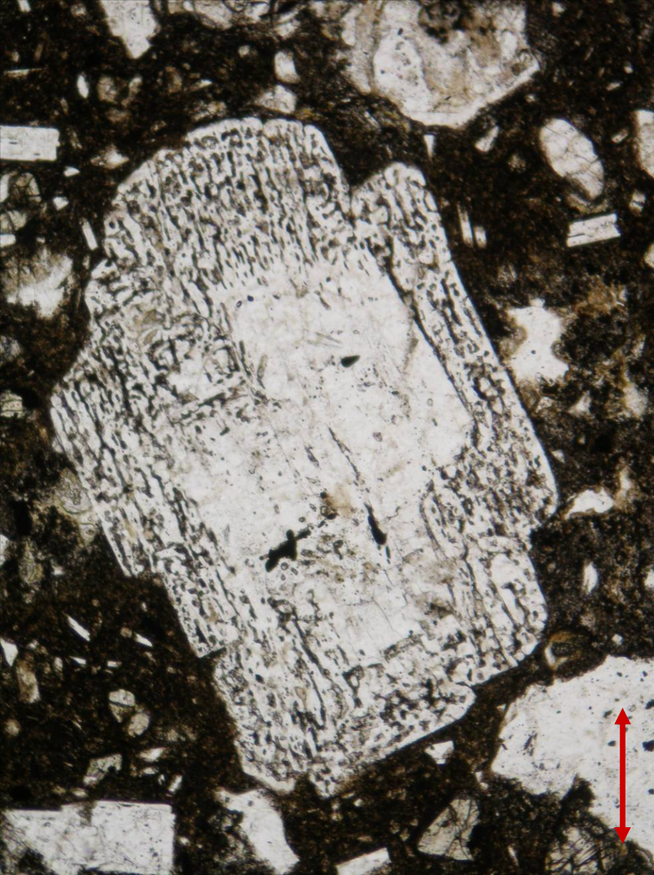
Plagioclase phenocryst (with hyaline matrix included in the rim) in andesite from Streda nad Bodrogom, Slovakia; PPL (left) and XPL (right). Width of fields of view is ca. 2.2 mm. Photo: JiZi.
