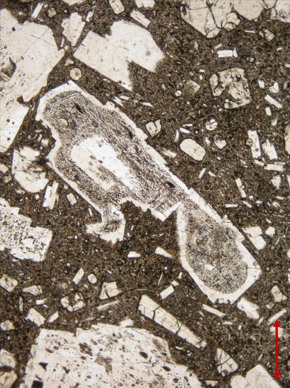
Plagioclase phenocrysts (with a sieve texture) in basalt or basaltic trachyandesite from Byšta, Slovakia; PPL (left) and XPL (right). Width of fields of view is ca. 2.0 mm. Photo: JiZi.
