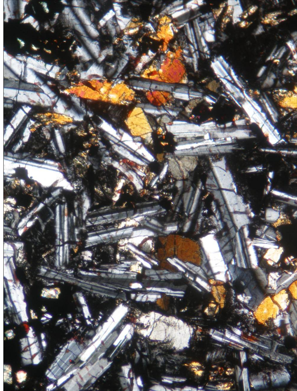
Plagioclase and pyroxene in palaeobasalt from Studenec, the Czech Republic; PPL (left) and XPL (right). Width of fields of view is ca. 1.7 mm. Photo: JiZi.
