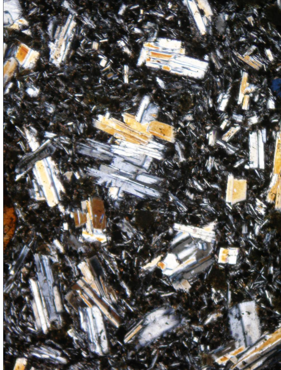
Plagioclase phenocrysts in andesite from Bánov, the Czech Republic; PPL (left) and XPL (right). Width of fields of view is ca. 1.5 mm. Photo: JiZi.
