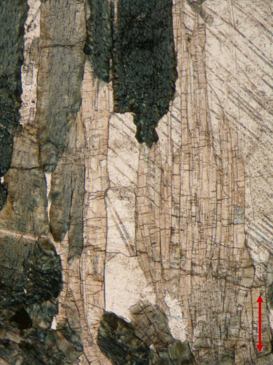
Tourmaline of the schorl-dravite series in a hydrothermal tourmaline-calcite vein from Chabičov, the Czech Republic; PPL (left) and XPL (right). Width of fields of view is ca. 1.7 mm. Photo: JiZi.
