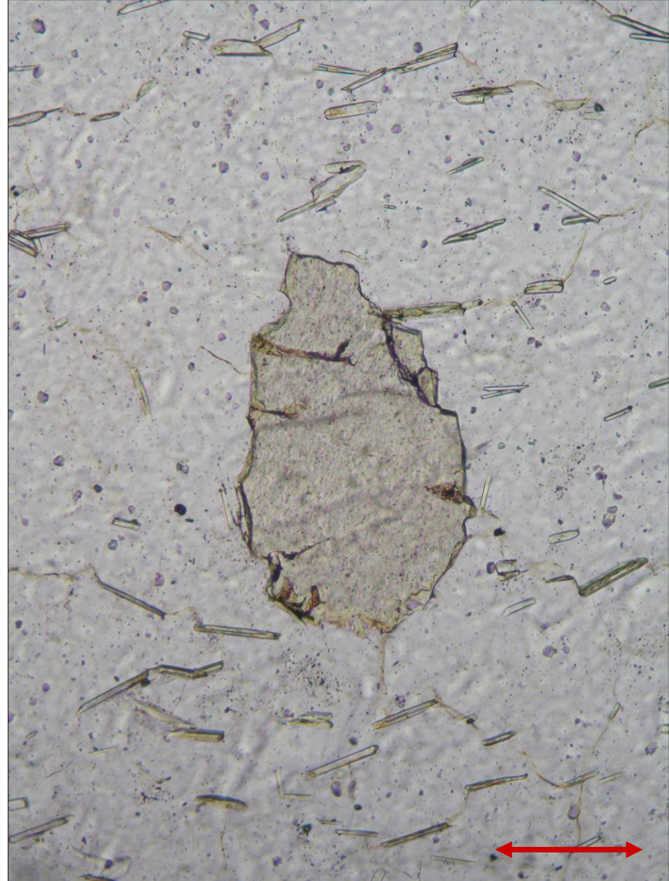
Strong pleochroism of tourmaline-schorl in quartzite from Petrov nad Desnou, the Czech Republic; PPL. Width of fields of view is ca. 0.8 mm. Photo: JiZi.
