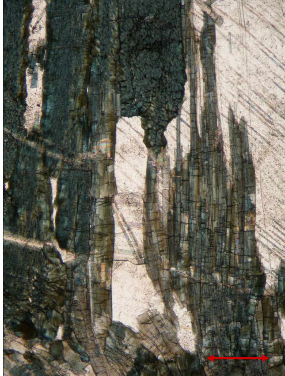
Strong pleochroism of tourmaline of the schorl-dravite series in a hydrothermal tourmaline-calcite vein from Chabičov, the Czech Republic; PPL. Width of fields of view is ca. 1.7 mm. Photo: JiZi.
