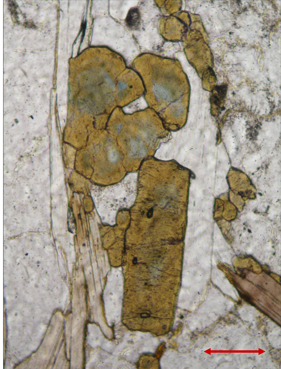
Color zoning and strong pleochroism of tourmaline in mica schist from Kovářová, the Czech Republic; PPL. Width of fields of view is ca. 0.7 mm. Photo: JiZi.
