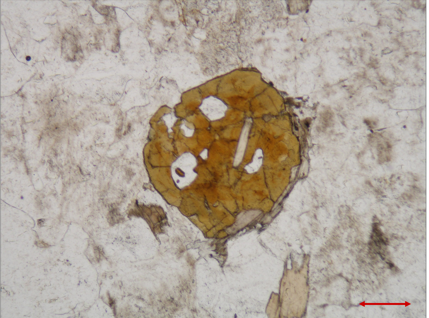
Tourmaline in orthogneiss from Hluboká, the Czech Republic; PPL. Width of the field of view is ca. 1.8 mm. Photo: JiZi.
