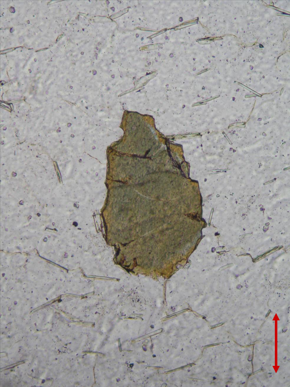
Strong pleochroism of tourmaline-schorl in quartzite from Petrov nad Desnou, the Czech Republic; PPL. Width of fields of view is ca. 0.8 mm. Photo: JiZi.
