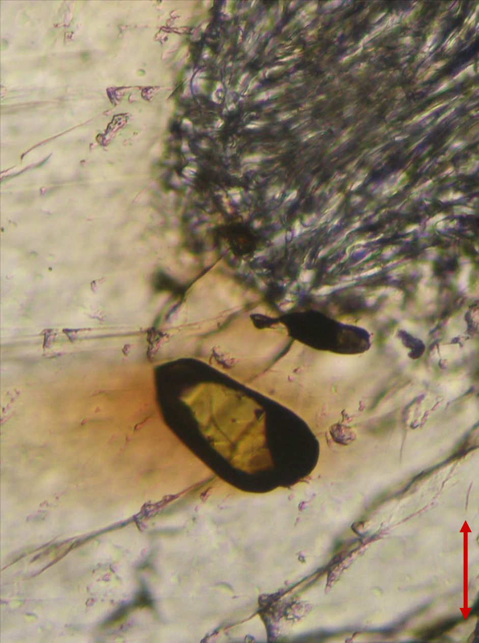
Rutile inclusions in clinopyroxene (omphacite) in eclogite from Borek, the Czech Republic; PPL (left) and XPL (right). Width of fields of view ca is. 0.3 mm. Photo: JiZi.
