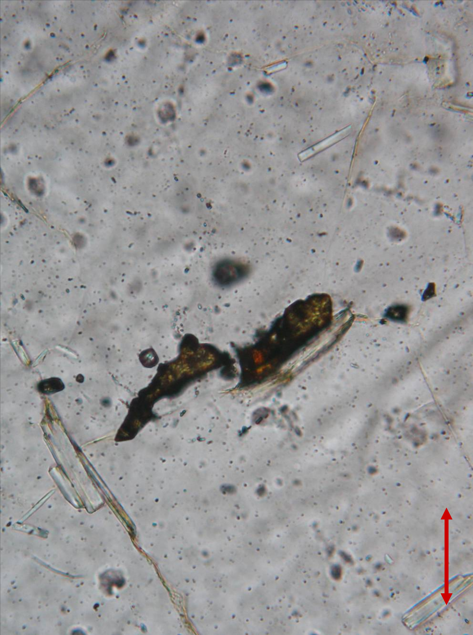
Rutile in quartzite from Petrov nad Desnou, the Czech Republic; PPL (left) and XPL (right). Width of fields of view is ca. 0.3 mm. Photo: JiZi.
