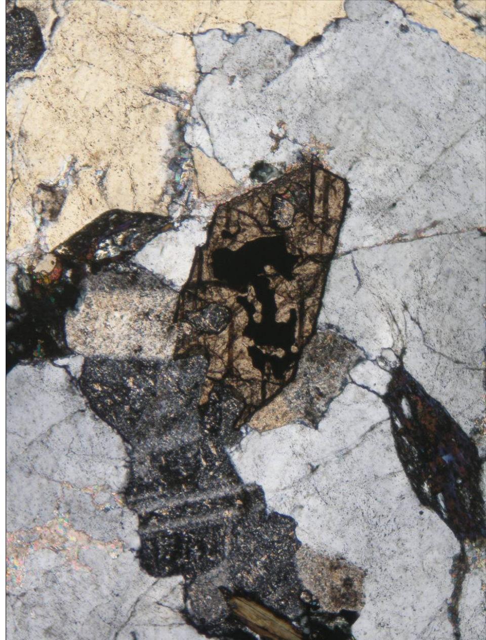
Titanite with opaque inclusions in granodiorite from Blansko, the Czech Republic; PPL (left) and XPL (right). Width of fields of view is ca. 1.5 mm. Photo: JiZi.
