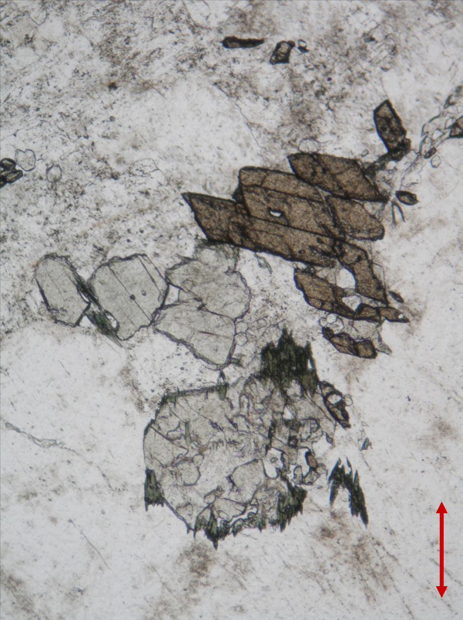
Titanite and diopside-hedenbergite in pegmatite from Žulová, the Czech Republic; PPL (left) and XPL (right). Width of fields of view is ca. 2.1 mm. Photo: JiZi.
