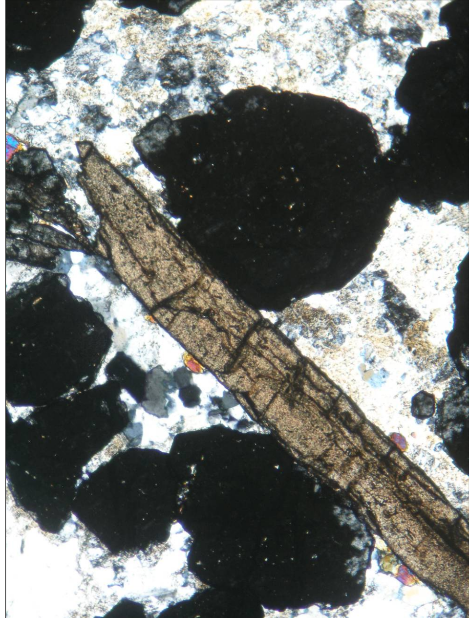
Titanite and garnet in metamanganolite from Vernířovice, the Czech Republic; PPL (left) and XPL (right). Width of fields of view is ca. 2.0 mm. Photo: JiZi.
