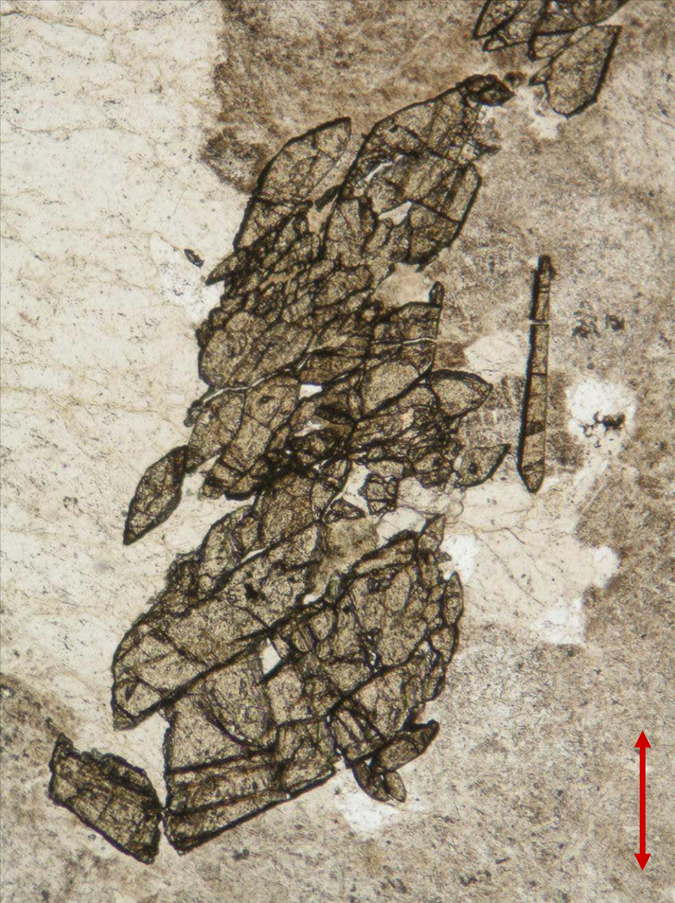
Titanite with quartz and altered feldspars in pegmatite from Supíkovice, the Czech Republic; PPL (left) and XPL (right). Width of fields of view is ca. 1.6 mm. Photo: JiZi.
