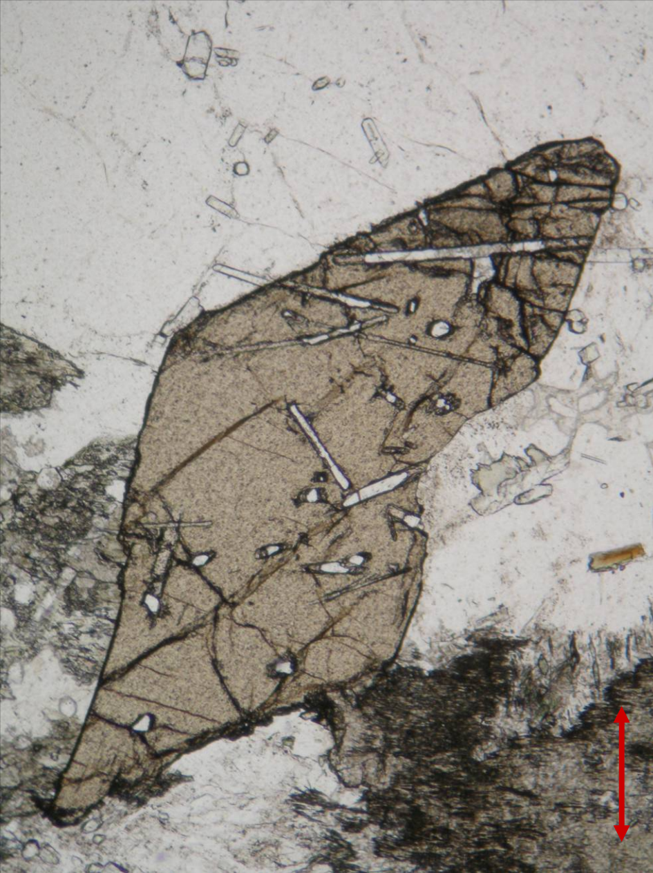
Titanite with apatite inclusions in pegmatite from Žulová, the Czech Republic; PPL (left) and XPL (right). Width of fields of view is ca. 2.0 mm. Photo: JiZi.
