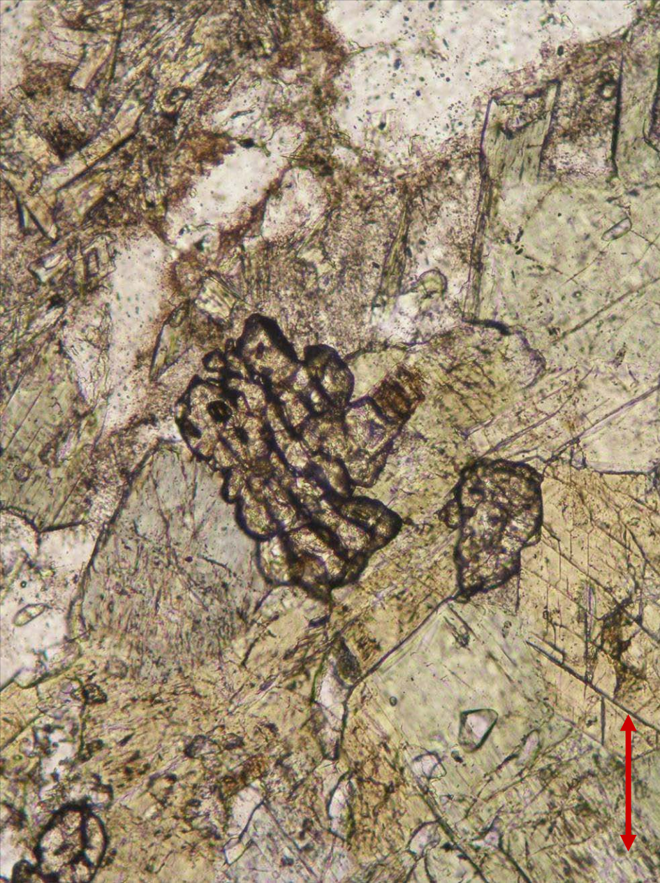
Titanite in garnet amphibolite from Petříkov, the Czech Republic; PPL (left) and XPL (right). Width of fields of view is ca. 0.6 mm. Photo: JiZi.
