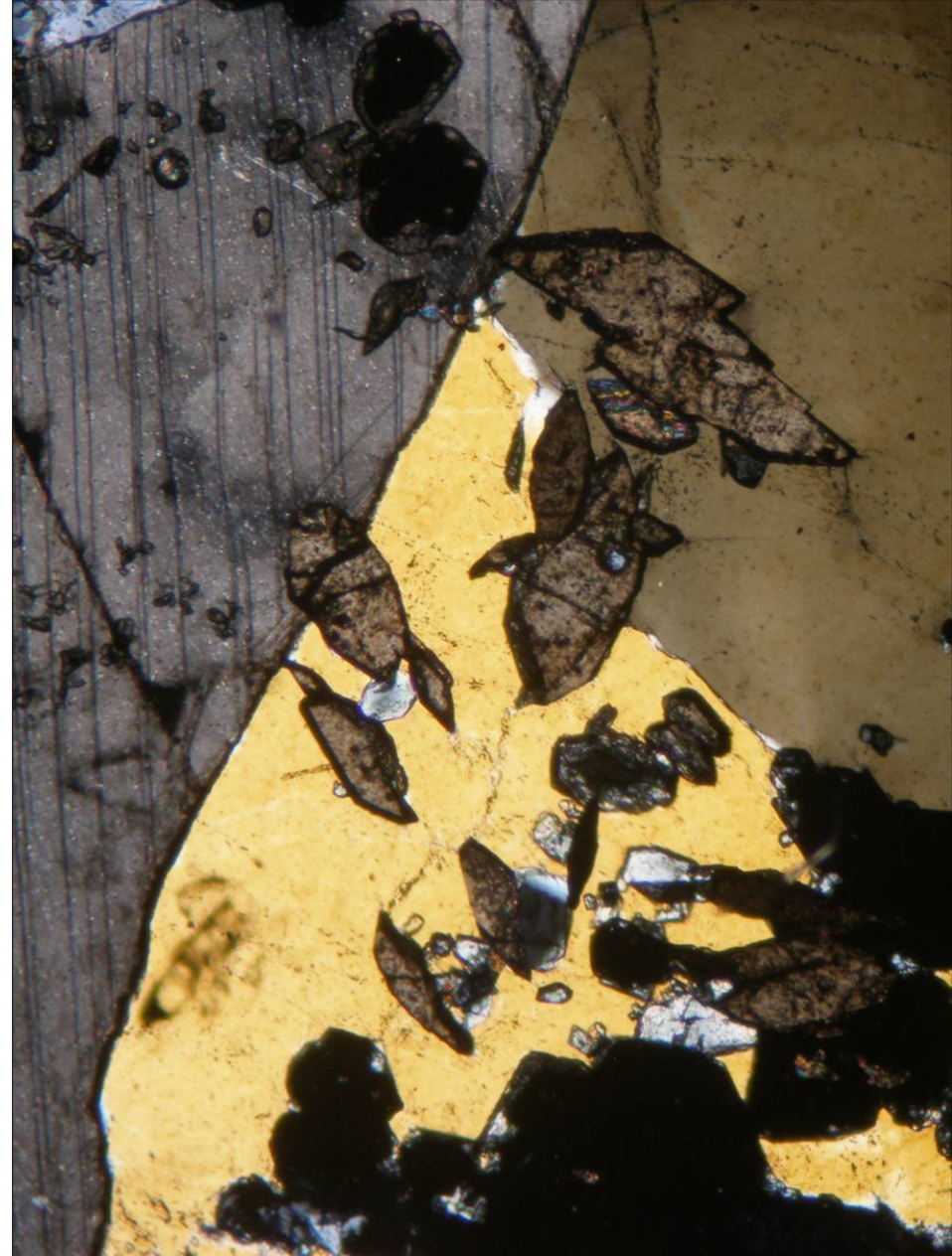
Titanite, garnet, calcite and quartz in skarn from Mirošov, the Czech Republic; PPL (left) and XPL (right). Width of fields of view is ca. 1.6 mm. Photo: JiZi.
