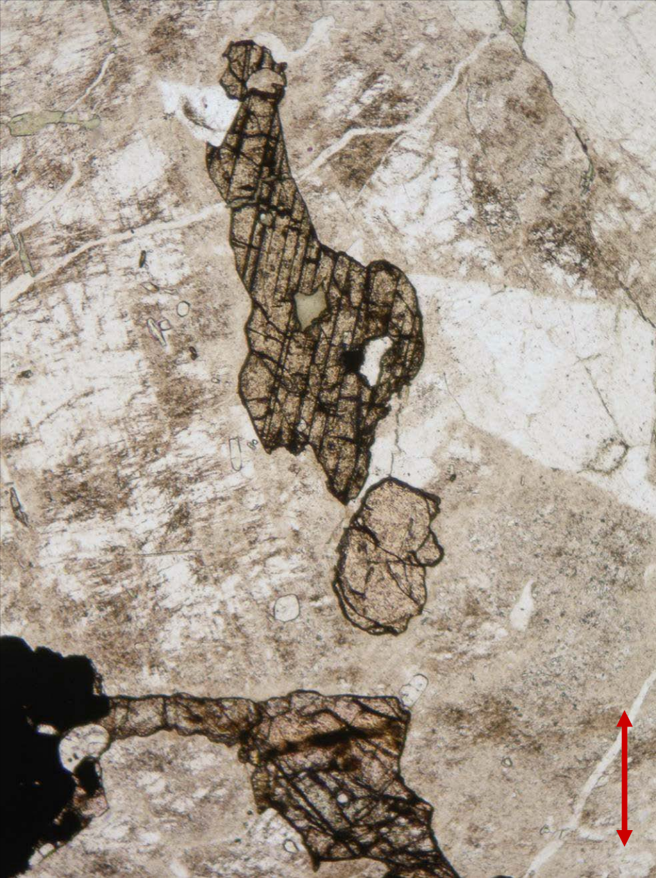
Titanite in granodiorite from Brno-Obřany, the Czech Republic; PPL (left) and XPL (right). Width of fields of view is ca. 1.7 mm. Photo: JiZi.
