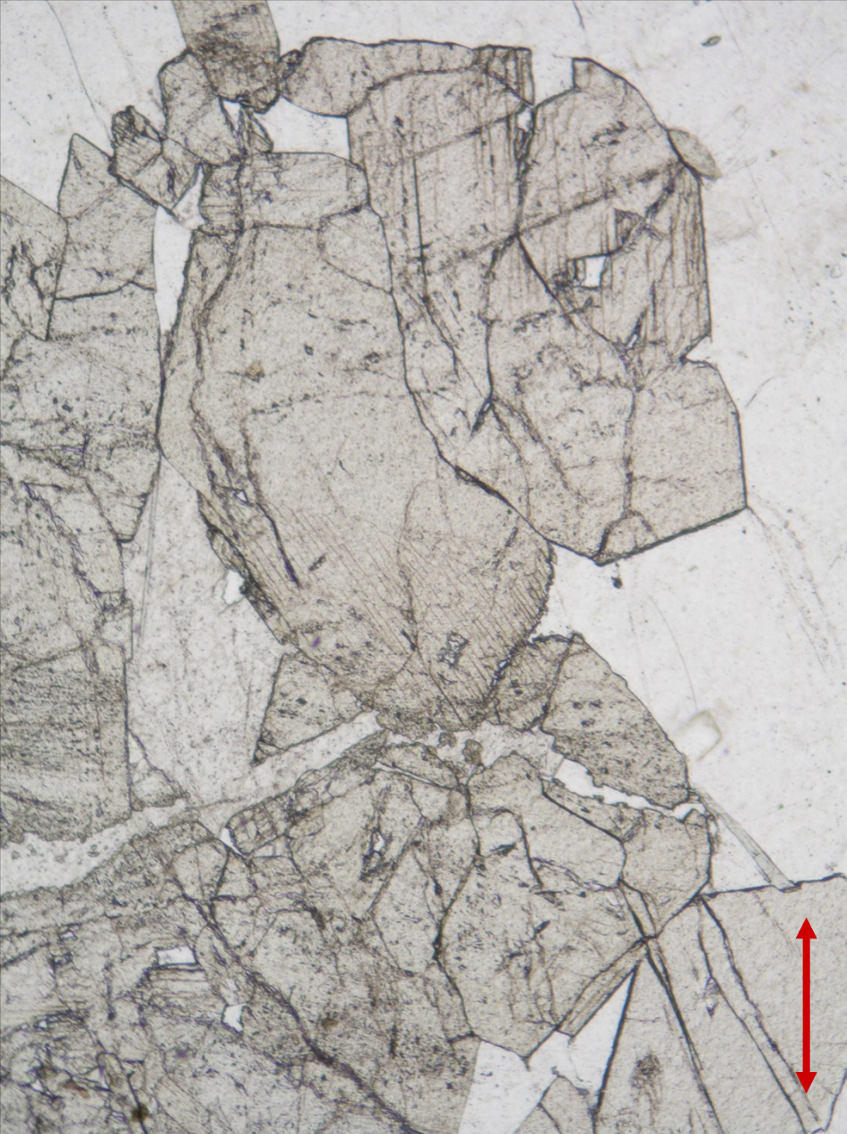
Epidote, quartz and calcite in the Alpine-type vein from Krásné near Hraběšice, the Czech Republic; PPL (left) and XPL (right). Width of fields of view is ca. 1.7 mm. Photo: JiZi.
