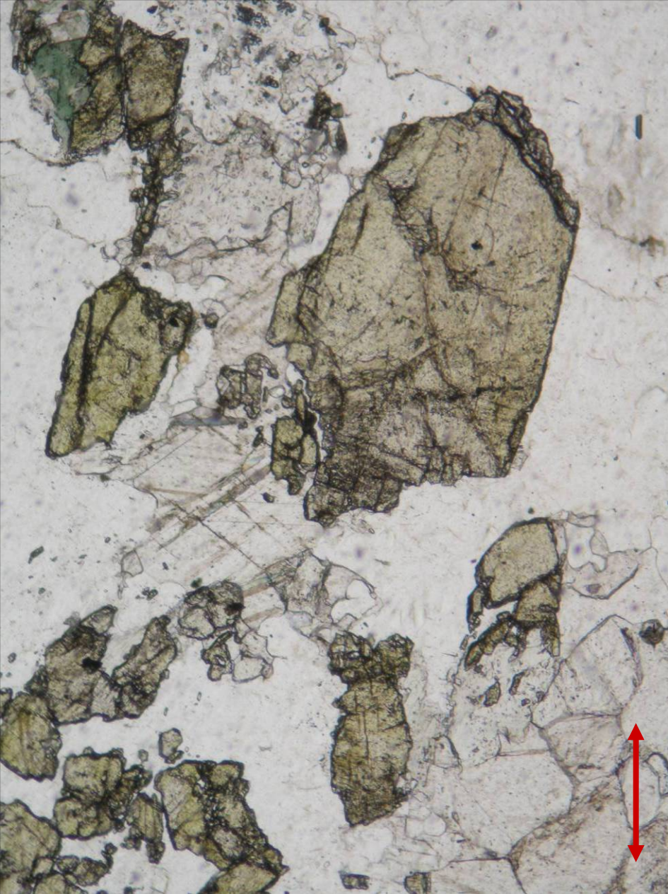
Epidote in a quartz-calcite band in greenschist from Drakov, the Czech Republic; PPL (left) and XPL (right). Width of fields of view is ca. 1.8 mm. Photo: JiZi.
