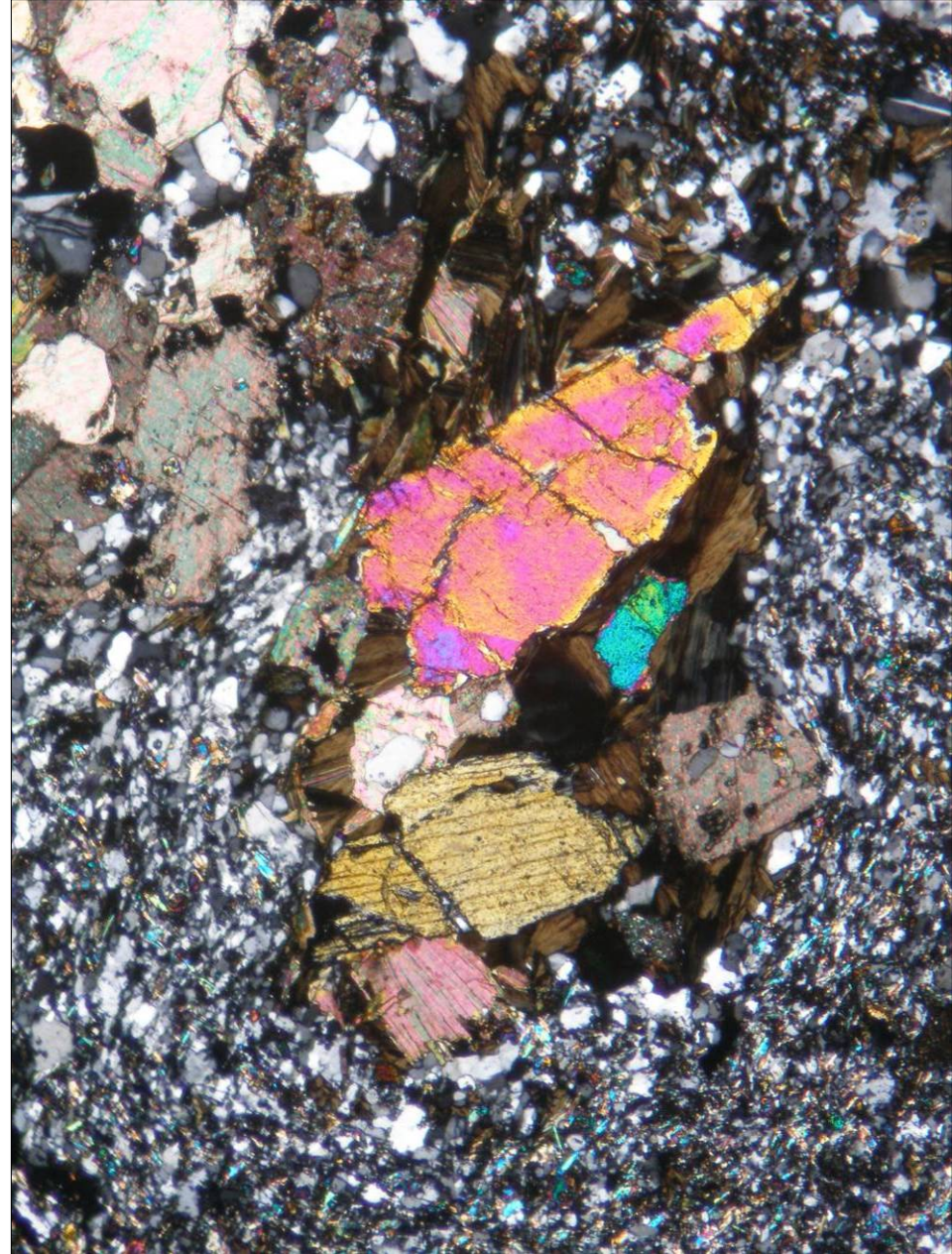
Epidote and chlorite in greenschist from Drakov, the Czech Republic; PPL (left) and XPL (right). Width of fields of view is ca. 1.8 mm. Photo: JiZi.
