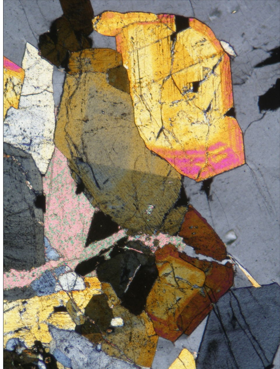
Epidote, quartz and calcite in the Alpine-type vein from Krásné near Hraběšice, the Czech Republic; PPL (left) and XPL (right). Width of fields of view is ca. 1.7 mm. Photo: JiZi.
