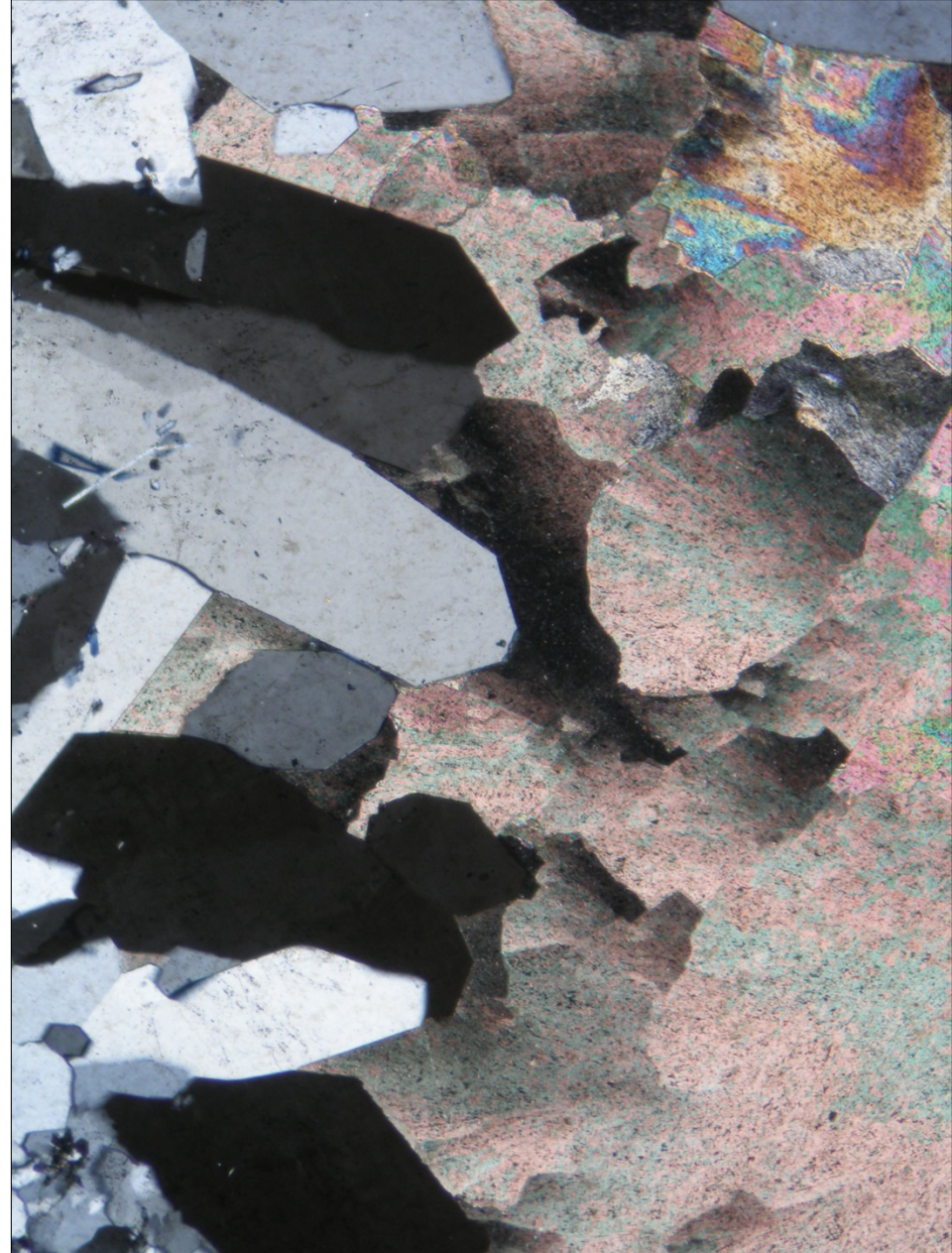
Quartz and carbonate of the dolomite-ankerite series in hydrothermal vein from Hrabůvka, the Czech Republic; PPL (left) and XPL (right). Width of fields of view is ca. 1.6 mm. Photo: JiZi.
