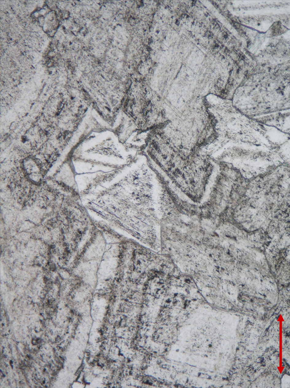
Zoning of dolomite-ankerite in a hydrothermal vein from Hrabůvka, the Czech Republic; PPL (left) and XPL (right). Width of fields of view is ca. 1.7 mm. Photo: JiZi.
