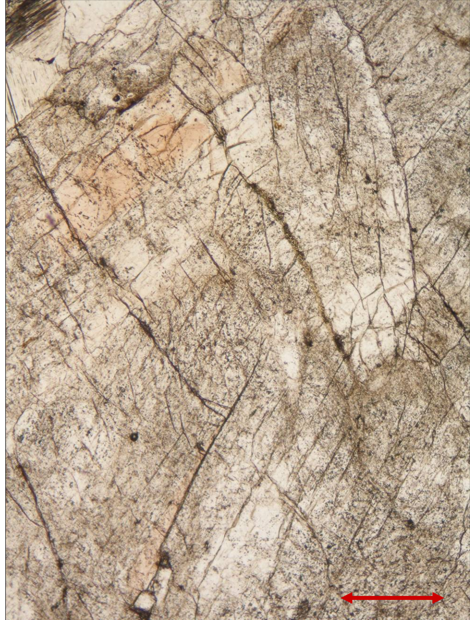
Pleochroism of andalusite in pegmatite from Dolní Bory, the Czech Republic; PPL. Width of fields of view is ca. 2.2 mm. Photo: JiZi.
