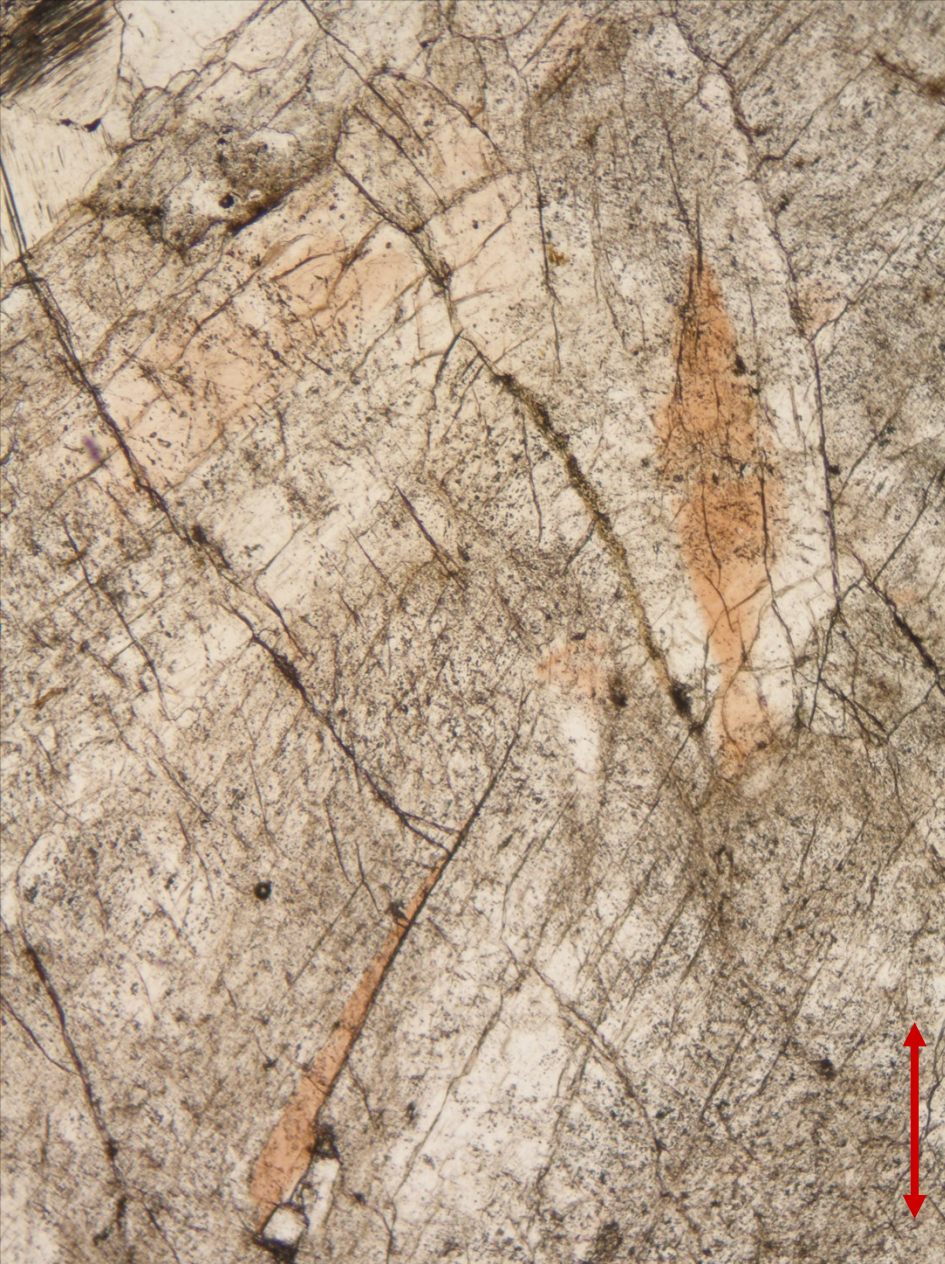
Pleochroism of andalusite in pegmatite from Dolní Bory, the Czech Republic; PPL. Width of fields of view is ca. 2.2 mm. Photo: JiZi.
