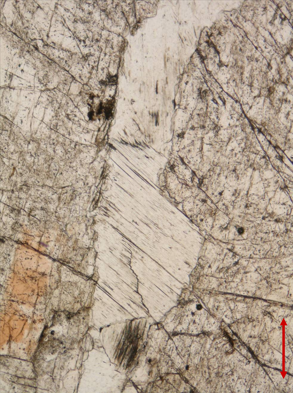
Andalusite and muscovite in pegmatite from Dolní Bory, the Czech Republic; PPL (left) and XPL (right). Width of fields of view is ca. 2.2 mm. Photo: JiZi.
