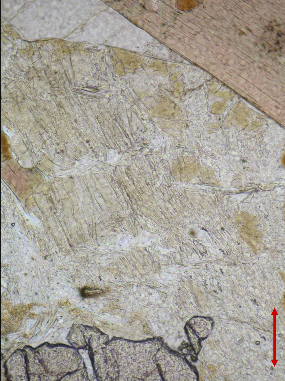
Cordierite (strongly pinitized) in gneiss from the Českomoravská vrchovina Highlands, the Czech Republic; PPL (left) and XPL (right). Width of fields of view is ca. 0.9 mm. Photo: JiZi.
