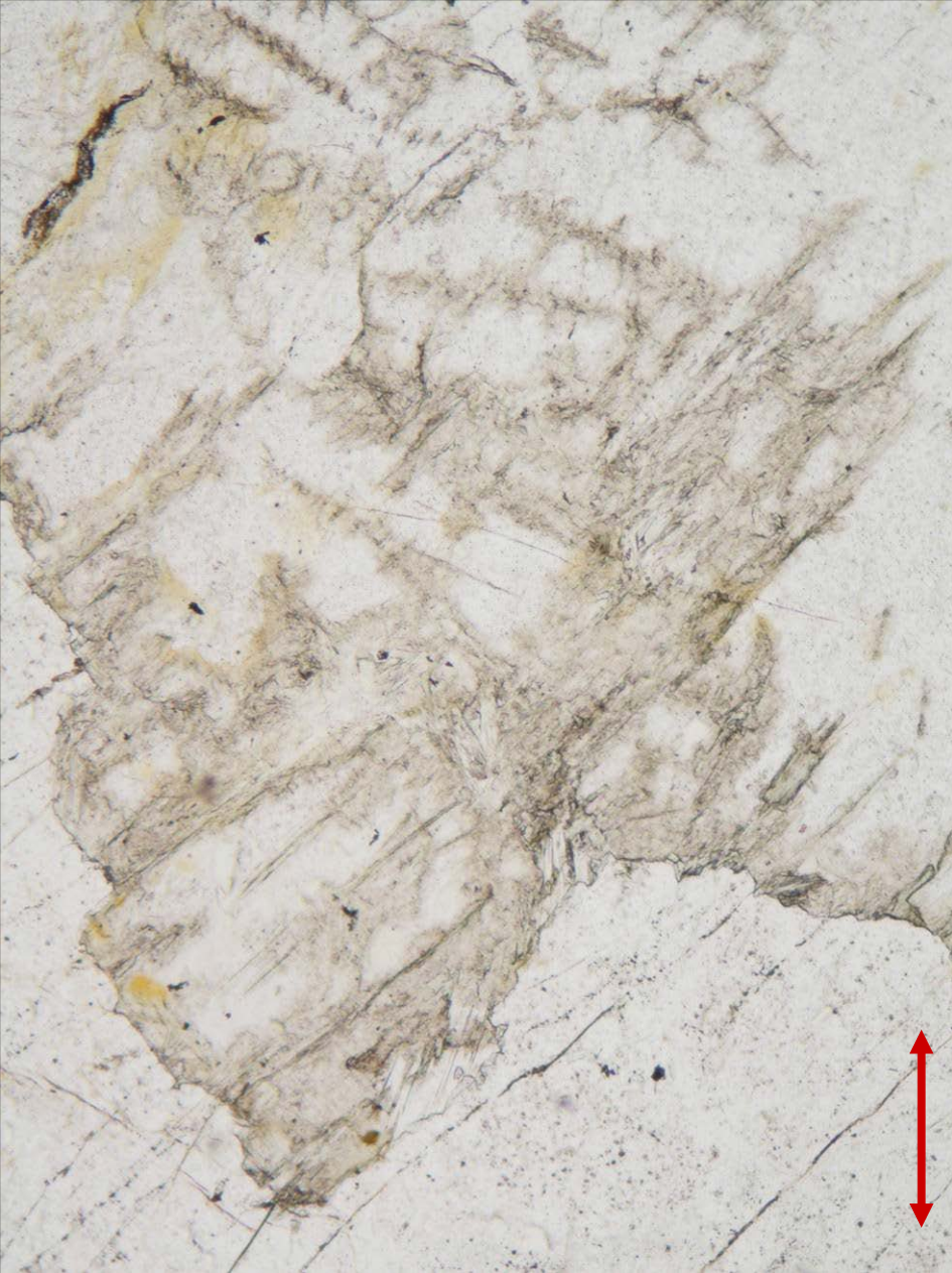
Cordierite (partly pinitized) in gneiss from Horní Bory, the Czech Republic; PPL (left) and XPL (right). Width of fields of view is ca. 1.8 mm. Photo: JiZi.
