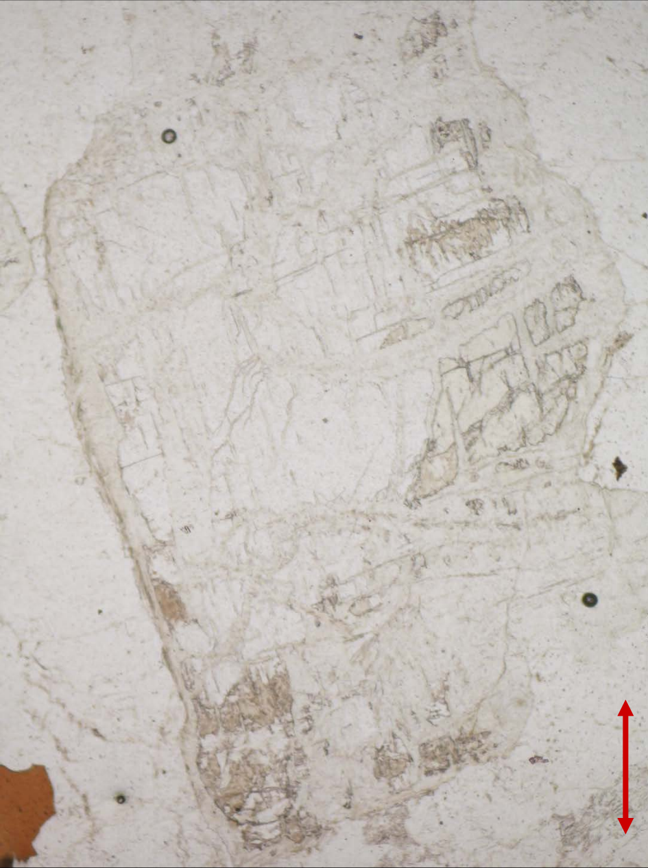
Cordierite (partly pinitized) in gneiss from the Českomoravská vrchovina Highlands, the Czech Republic; PPL (left) and XPL (right). Width of fields of view is ca. 2.2 mm. Photo: JiZi.
