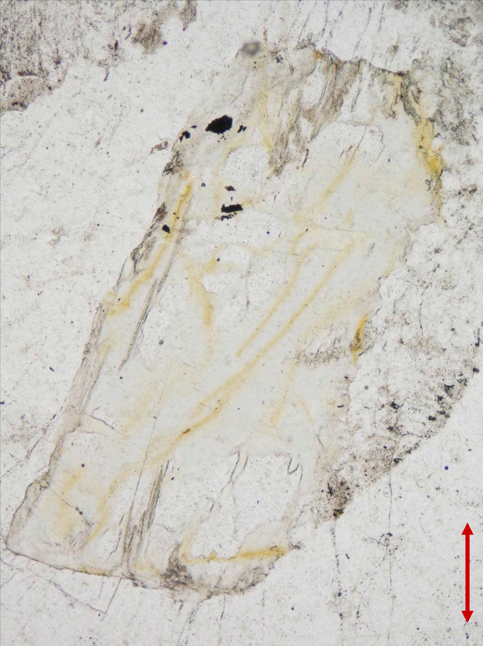
Cordierite in gneiss from Horní Bory, the Czech Republic; PPL (left) and XPL (right). Width of fields of view is ca. 1.8 mm. Photo: JiZi.
