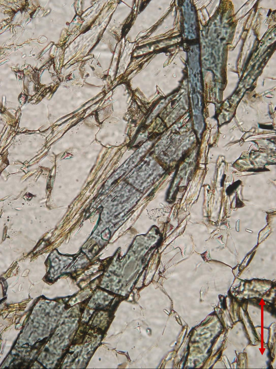
Chloritoid in phyllite from Nový Malín, the Czech Republic; PPL (left) and XPL (right). Width of fields of view is ca. 0.4 mm. Photo: JiZi.
