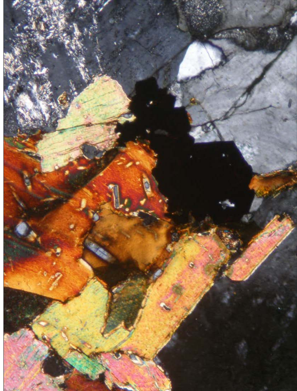
Magnetite in syenite from Tasov, the Czech Republic; PPL (left) and XPL (right). Width of fields of view is ca. 1.4 mm. Photo: JiZi.
