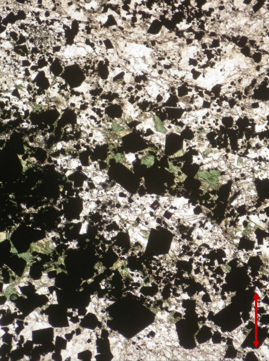
Magnetite, chlorite and calcite in iron ore from Horní Moravice, the Czech Republic; PPL (left) and XPL (right). Width of fields of view is ca. 2.2 mm. Photo: JiZi.
